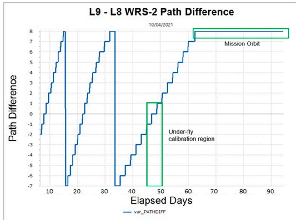
Figure 4. Landsat 9 offset from Landsat 8 in WRS-2 path difference.
