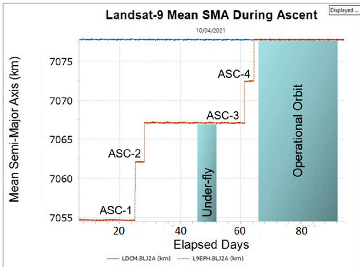
**Figure 3.** Landsat 9 Semi-major Axis versus Elapsed Days for launch.
