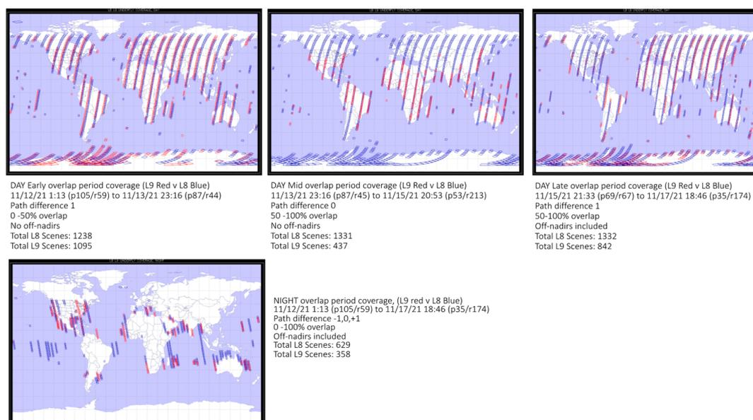
**Figure 9.** Landsat 9 and Landsat 8 Path(P)/Rows(R) Acquired During the Tandem flying (Day and Night).
