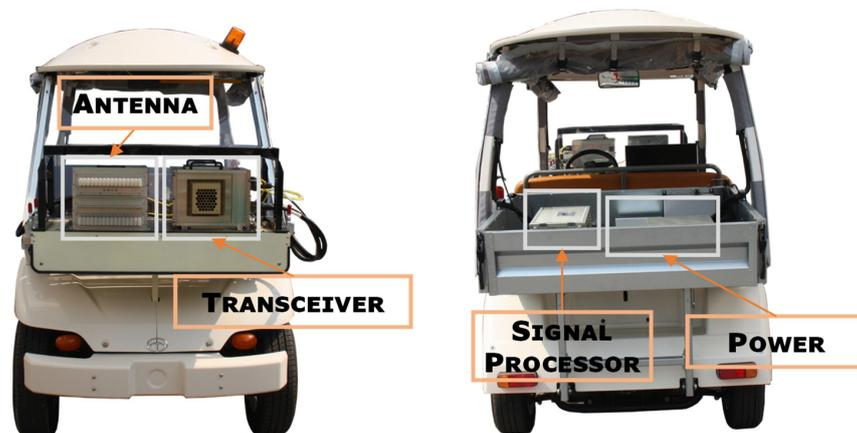
**Figure 16.** Test vehicle (Front and Back view).
