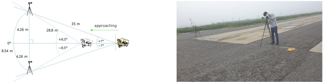
Figure 23. Test setup for measuring the angular resolution.
