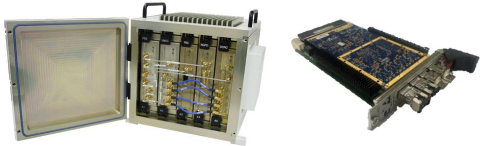
**Figure 15.** Digital correlator (left) and DSP signal processing board (right).
