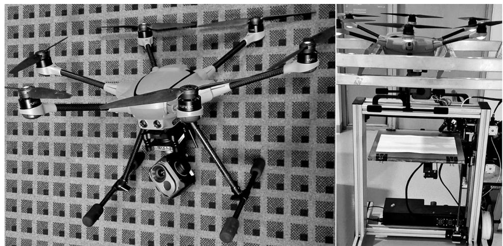
**Figure 2.** H520 drone with the E10T camera. The drone is attached to the radiometric calibration over the heated bed of the Omni3d Factory 1.0 printer.
