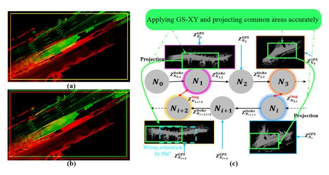
**Figure 6.** (a) Two nodes merged wrongly by PhC. (b) Correct merging by GS-XY showing the correct position of the common area in each node. (c) GS-framework in the Z plane applied on elevation images based on projected areas by GS-XY.
