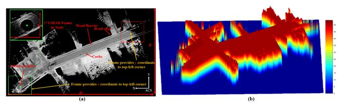
**Figure 3.** Accurate node strategy. (a) Intensity image to represent road surface at 0.3 m in the Z-direction with surrounding environments and top-left corner identification tactic. (b) Elevation image.
