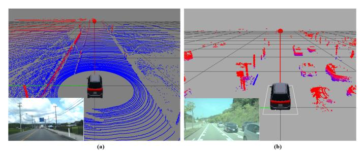
**Figure 2.** (a) Featureless wide road in the Z-direction. (b) Preventing static features to be encoded at a traffic signal by stopped cars.
