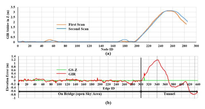
**Figure 12.** (a) Standard deviation of the GIR system in the Z plane showing unstable accuracy along elevation images inside the Yamate Tunnel. (b) Large altitudinal differences between common areas in GIR elevation images (red profile) and the significant small differences after applying GS-Z (green profile). The dotted lines refer to edges in Figure 13.
