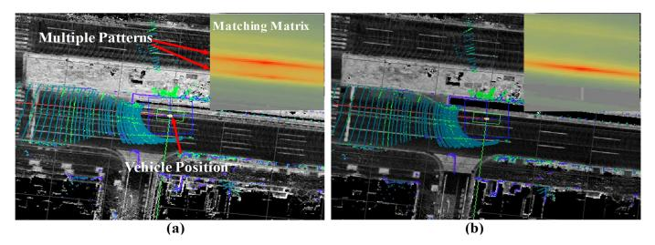
**Figure 1.** (a) Ghosting effects (duplication of road landmarks because of scanning the segment twice with different positioning accuracies by GNSS/INS-RTK) in the map and multiple matching patterns with the observation point cloud. (b) Identical map without ghosting and the corresponding matching result.
