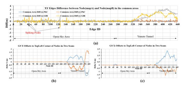
**Figure 9.** (a) Loop-closure edges (coordinate difference) of the common areas between two scans in x and y directions obtained by GNSS/INS-RTK system and phase correlation on the node images. (b) The proposed GS-XY's Y-offsets to top-left corners of nodes in the first and second scans. (c) X-offsets to two scans.
