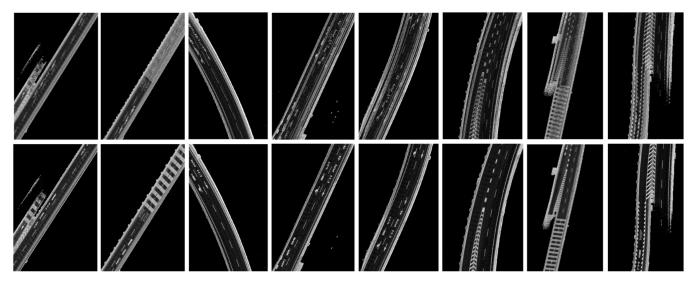
**Figure 10.** Wrong combined node images inside the Yamate Tunnel by GIR (first row) and accurate combination by GS-XY framework (bottom).
