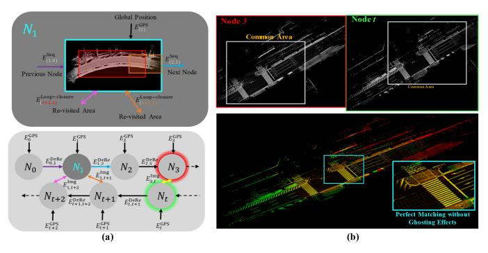
**Figure 5.** (a) Relationship between nodes in the XY plane and edge types of GS-XY cost function. (b) Applying PhC to merge two nodes (*N*3 and *Nt*) based on matching road landmarks with estimating common areas for loop-closure edges.
