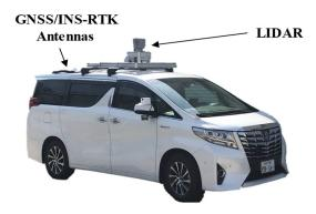
Figure 7. Experimental platform with sensor configurations.
