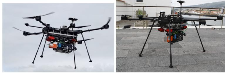
**Figure 6.** Hyperspectral imaging system mounted in the unmanned aircraft (Grifo-X).
