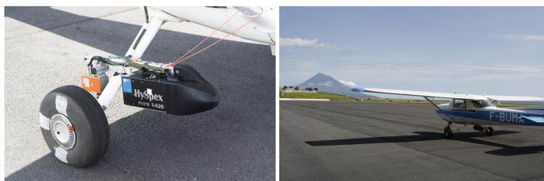
**Figure 5.** Hyperspectral imaging system mounted in the manned aircraft (F-BUMA).
