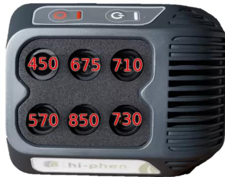
**Figure 1.** AIRPHEN camera composed of 6 sensors
