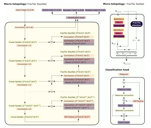
ResNet unit. The final layer of the decoder, as well as the output of the first convolution layer, are the inputs to the classification head.
