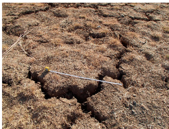
Figure A5. Soil cracks observed in Rashda village.
