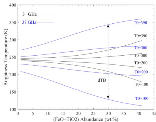
**Figure 2.** Change of simulated  $T_B$  with  $(\text{FeO}+\text{TiO}_2)$  abundance and surface temperature.
