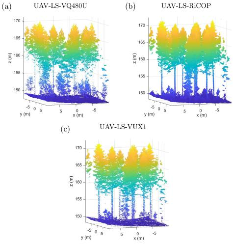
**Figure 8.** Point clouds of the sparse test site obtained with the different above-canopy flying UAV systems: (a) UAV-LS-VQ480U, (b) UAV-LS-RiCOP, and (c) UAV-LS-VUX1.
