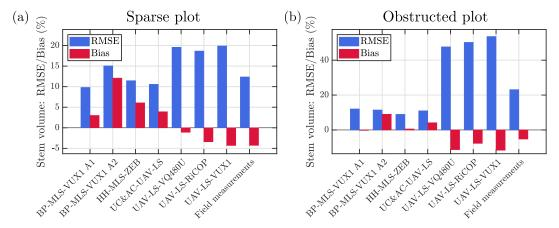
**Figure 13.** Relative bias and RMSE of stem volume estimation at the individual tree level for the different methods (**a**) in the sparse plot and (**b**) in the obstructed plot. BP, HH, and UC stand for backpack, handheld, and under-canopy, respectively. Note that the scales of the y axes are different in panels (**a**,**b**).
