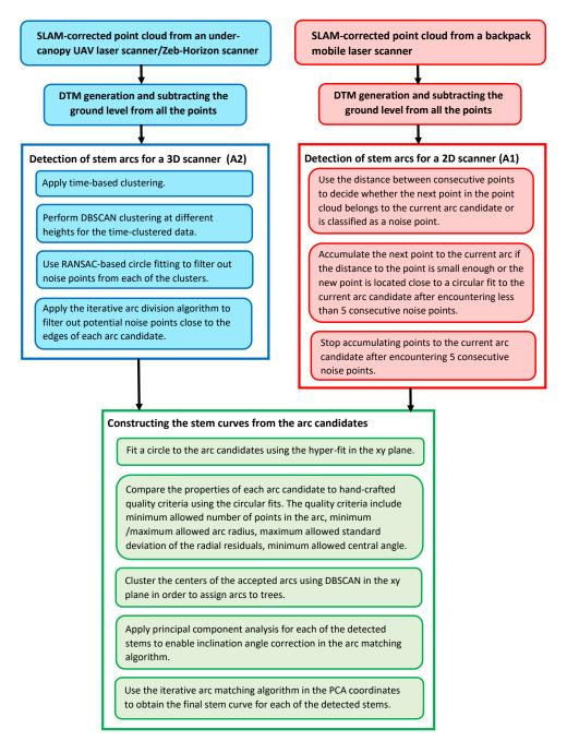
**Figure 6.** Flow chart of the stem curve extraction algorithm used for the backpack laser scanner, under-canopy UAV laser scanner, and handheld laser scanner. The algorithms are based on our previous work [13,14].
