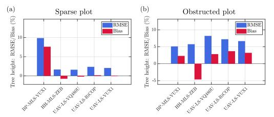
**Figure 11.** Relative bias and RMSE of tree height estimation at the individual tree level for the different methods (a) in the sparse plot and (b) in the obstructed plot. BP and HH stand for backpack and handheld, respectively. Note that the scales of the y axes are different in panels (a,b).
