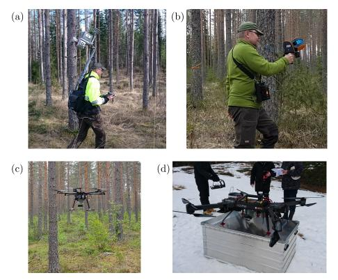
**Figure 3.** Photographs of (a) the backpack mobile laser scanning unit (BP-MLS-VUX1), (b) the handheld ZEB-Horizon laser scanner (HH-MLS-ZEB), (c) the under-canopy UAV laser scanning system (UC-UAV-LS), and (d) the RiCopter laser scanning system (UAV-LS-RiCOP).
