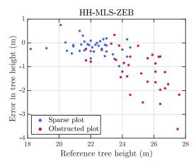
**Figure 12.** Error in the tree heights estimated from the point cloud collected with the handheld Zeb-Horizon scanner as a function of tree height. Note the increasing underestimation in the heights of trees taller than 25 m.
