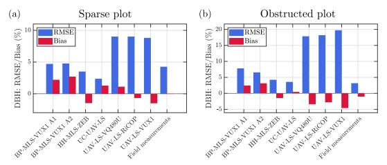
**Figure 9.** Relative bias and RMSE of DBH estimation at the individual tree level for the different MLS methods (a) in the sparse plot and (b) in the obstructed plot. BP, HH, and UC stand for backpack, handheld, and under-canopy, respectively. Note that the scales of the y axes are different in panels (a,b).
