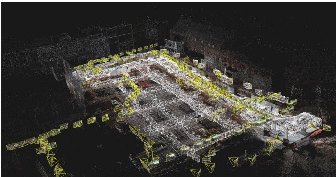
**Figure 1.** In the proposed method the alignment of recorded site images (white) is aided by the pre-registered accurate reference module (yellow).
