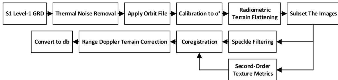
**Figure 3.** Schematic view of the Sentinel-1 pre-processing workflow.
