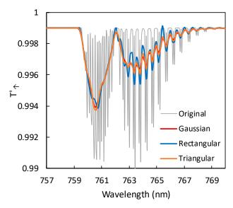
**Figure 9.** MODTRAN simulated up-welling transmittance convolved with Gaussian, Rectangular and Triangular instrument spectral response function (ISRF) with a full-width at half maximum (FWHM) of 0.31 nm and resampled with spectral interval of 0.155 nm. The FWHM of the original simulation (grey line) is  $1 \text{ cm}^{-1}$  (~0.06 nm at 760 nm), the sensor height is 25 m, the surface elevation is 1.5 km, the view zenith angle (VZA) is 25°, and the AOD<sub>550</sub> is 0.1.
