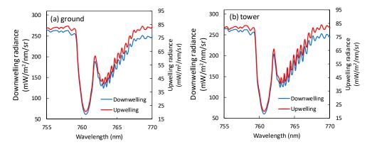
**Figure 10.** Downwelling and upwelling radiance at O<sub>2</sub>-A band measured on the ground and on the tower (without atmospheric correction) at 13:01 on 7 September 2018, at the Daman site.
