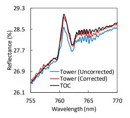
**Figure 6.** Comparison of the apparent reflectance spectra at  $O_2$ -A band measured on the ground and on the tower (with/without atmospheric correction) at 13:01 on 7 September 2018, at the Daman site.
