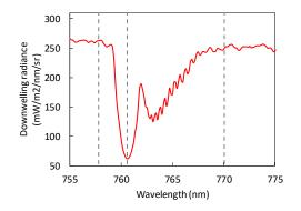
**Figure 4.** Illustration of the bands used in 3FLD method for solar-induced chlorophyll fluorescence (SIF) retrieval in this study. The vertical dash lines shows the spectral position of the bands at the left of, inside, and at the right of the O<sub>2</sub>-A absorption feature.
