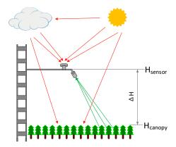
Figure 3. Illustration of the tower-based automatic spectral observation system.
