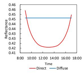
**Figure 8.** Simulated diurnal variation in direct and diffuse radiation canopy reflectance at 760.6 nm using the Soil Canopy Observation, Photochemistry and Energy fluxes (SCOPE) model for an LAI of 4 and spherical leaf inclination distribution function (LIDF).
