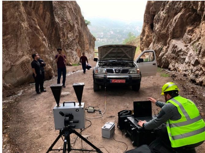
Figure 3. Radar deployment under the Veresk Bridge.
