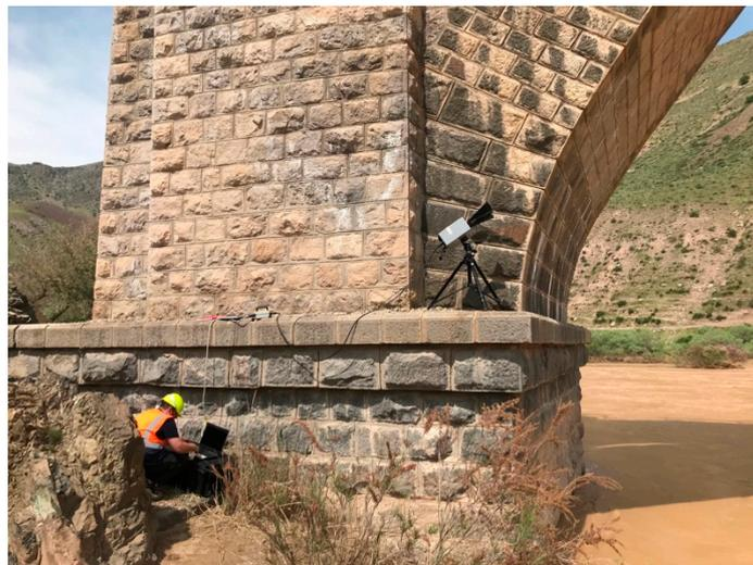
Figure 4. Radar installation at the Kaflan-Kuh Bridge.
