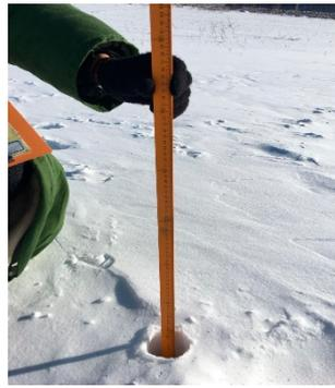
**Figure 8.** A wooden ruler for measuring snow depth.
