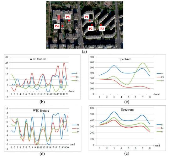
**Figure 12.** Comparisons of WIC and spectral features. (a) The selected five pixels (P1, P4, and P5 are building pixels; P2 and P3 are shadow and vegetation pixel respectively); (**b**,**c**) WIC and spectral feature curves of P1, P2, and P3; and (**d**,**e**) WIC and spectral feature curves of P1, P4, and P5.
