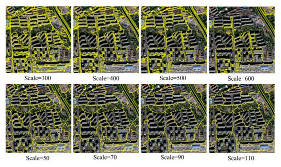
**Figure 13.** The segmentation results using traditional multiresolution segmentation (MRS) in e-Cognition software (the top images are the results of the original image, while the bottom images are the results of the WIC feature image).
