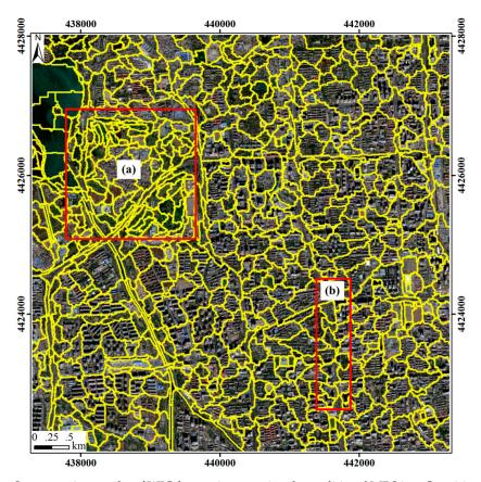
**Figure 15.** Segmentation results of WIC feature image using the traditional MRS in e-Cognition software with scale = 90. (a) Large UFZs are over-segmented seriously; and (b) many UFZs cross roads.
