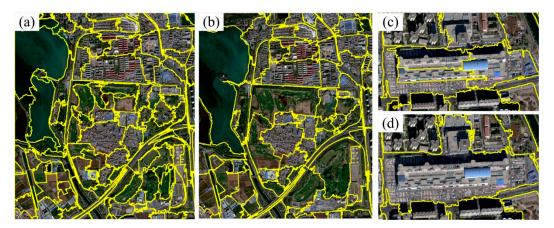
**Figure 18.** The effectiveness of scale-adaptive method. (**a**,**c**) are the results of fixed-scale method; (**b**,**d**) are the results of adaptive-scale method.
