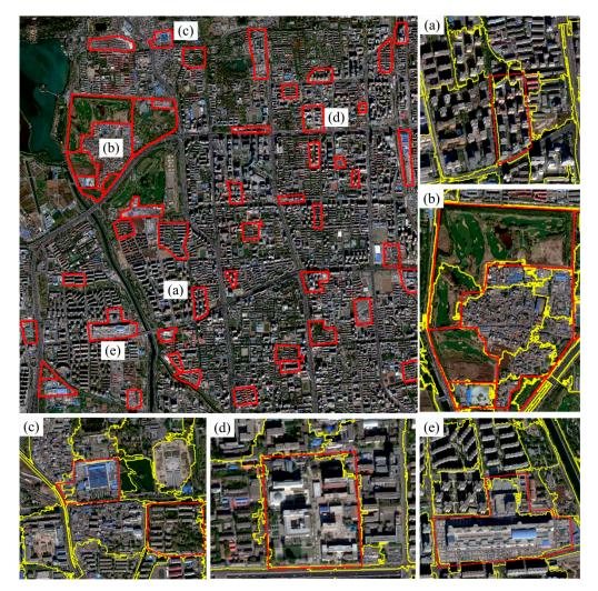
**Figure 8.** The reference data and the comparison with segmentation results (the red lines are reference data and the yellow lines are segmentation results). (a) Residential districts; (b) shantytowns and parks; (c) industrial zones and residential districts; (d) campuses; and (e) commercial zones.
