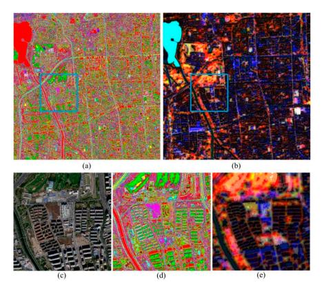
**Figure 6.** The ISODATA classified image and WIC feature image. (a) The ISODATA classified image; (b) the WIC feature image (R, G, and B assigned with feature bands 1, 2, and 3 respectively); (c) amplified view of original image of blue rectangles in (a,b); (d) amplified view of ISODATA classified image; (e) amplified view of WIC feature image.
