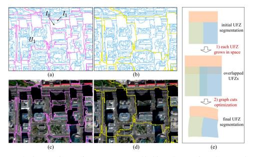
**Figure 4.** The diagram of energy function construction (the blue polygons refer to the image objects segmented by step (2); the purple polygons refer to the initial UFZs segmented by step (3), while the yellow polygons refer to the final UFZs). (a) Image objects and initial UFZs; (b) image objects and final UFZs; (c) initial UFZs; (d) final UFZs; and (e) brief illustration of graph cuts optimization.
