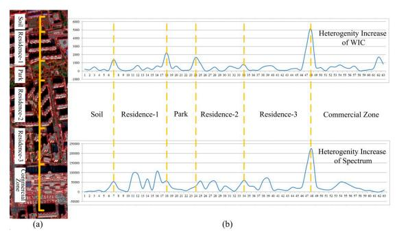
**Figure 14.** The heterogeneity increase of the object merging in MRS using the WIC and spectral features. (a) The objects crossed by the orange line are selected; and (b) the heterogeneity increase of the WIC and spectral features.
