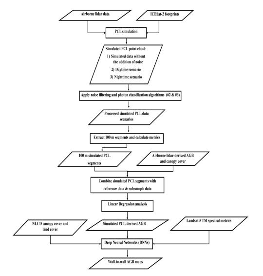
Figure 3. Workflow for mapping AGB using simulated ICESat-2 and Landsat data.
