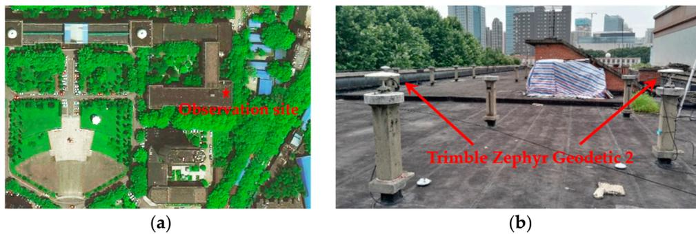
**Figure 1.** Observational environment and GNSS antennas used in the experiments at SGG building of Wuhan University. (a) shows the observation site on the roof of SGG building, and (b) shows the Trimble Zephyr Geodetic 2 antenna and the short baseline configuration.
