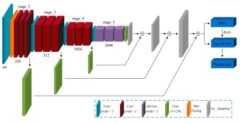
Figure 1. Architecture of the deformable Faster CNN with three TCBs.
