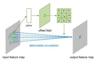
**Figure 2.** Illustration of  $3 \times 3$  deformable convolution.
