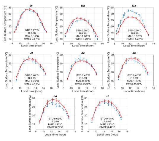
**Figure 4.** Diurnal cycle of UAV-based LST (blue dashed line) versus *in situ* temperature as measured by Apogee sensors (red line) for the December (D1–D3) and January (J1–J5) campaigns, along with statistics including the *in situ* LST standard deviation (STD), correlation coefficient (R), mean absolute error (MAE) and root mean square error (RMSE).
