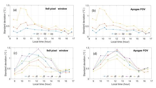
**Figure 3.** Standard deviation of diurnal UAV-based land surface temperature (LST) within  $9 \times 9$  pixels (90  $\times$  90 cm) (**a,c**) and Apogee field-of-view (FOV) windows (**b,d**) for the 3 stations (D1–D3) on 13 December 2016 and for the 5 stations (J1–J5) on 31 January 2017.
