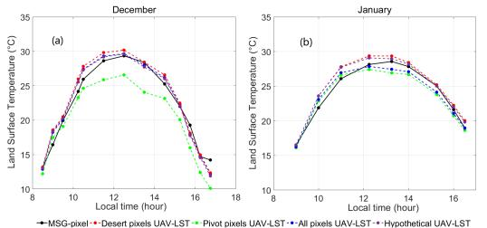
Figure 10. Diurnal Meteosat Second Generation (MSG)-based LST, UAV-based LST for all observed
