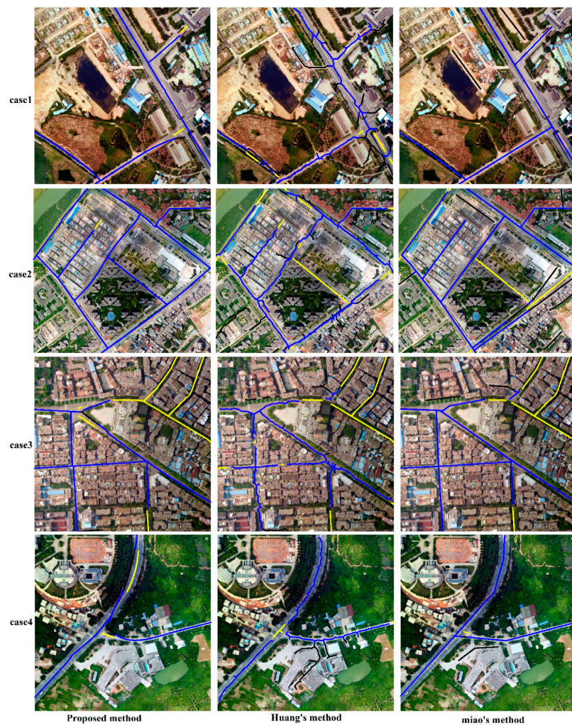
Figure 7. Comparison of the road centerline network extraction of different methods for the Guangzhou dataset. True positives are shown in blue, false positives in yellow, and false negatives in black.
