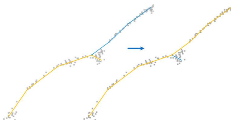
**Figure 5.** Example of branch connection refinement. Gray dots are scanned branch points, yellow and blue lines are connection lines. The right panel shows a more natural way of connection than the left.
