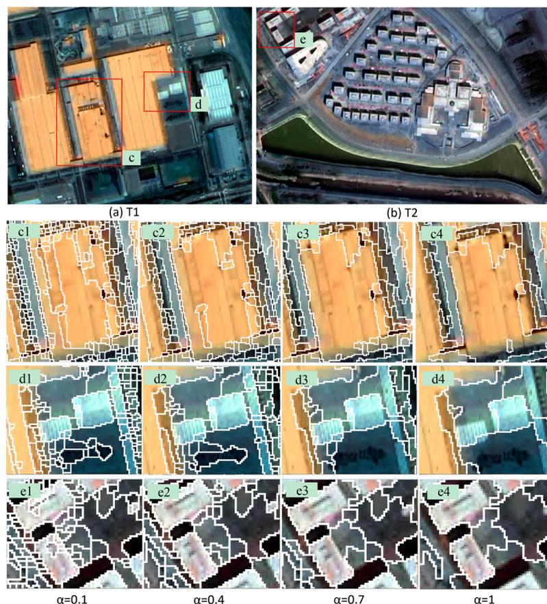
**Figure 5.** Segmentation results of urban subsets, where the parameter  $\alpha$  is set at 0.1, 0.4, 0.7 and 1 from left to right.
