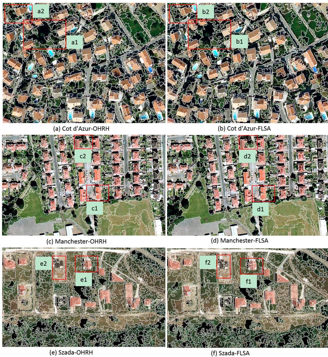
**Figure 18.** Segmentation results produced with the OHRH and FLSA methods, using the SZTAKI-INRIA building detection dataset.
