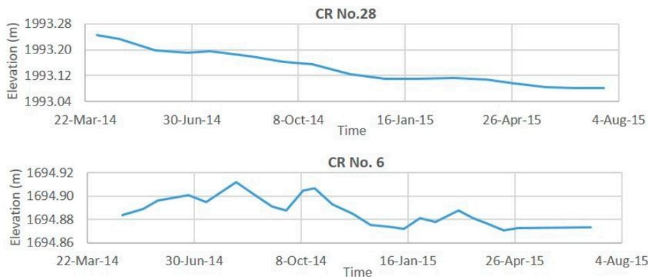
**Figure 10.** Linear and non-linearity behaviors of CRs. Elevation changes of CR28 and CR6 are derived by the GPS measurements.
