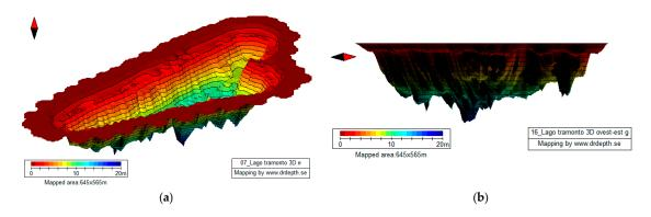
**Figure 4.** Tridimensional elaborations of Lago Tramonto in Gambulaga, Portomaggiore (FE, Italy): (a) 3D bathymetry; (b) 3D section West-East (using Hydrosynergy).
