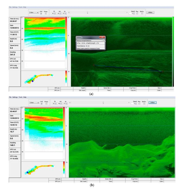
**Figure 7.** Visualization of the echo side scan sonar snap shots with Hum viewer software, in Lago Tramonto, Gambulaga, Portomaggiore (FE, Italy): (**a**) Bottom, down image and position with metrical reference of a big trunk; (**b**) Bottom, down image and position of anthropic traces.
