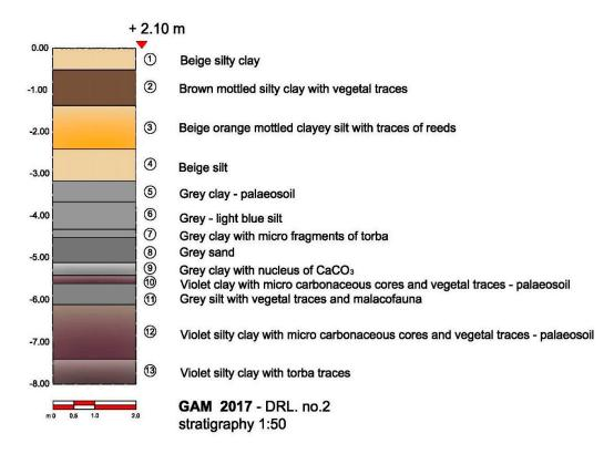
**Figure A2.** Graphic depiction of drilling No. 2 in 2017 in Lago Tramonto, Gambulaga, Portomaggiore (FE, Italy).
