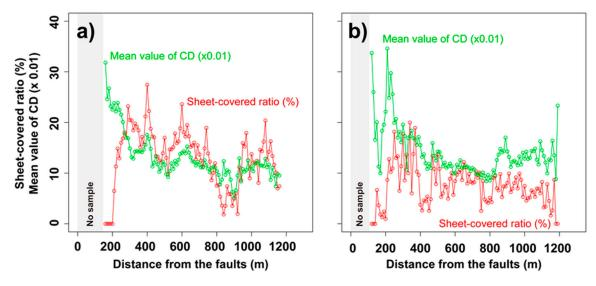
**Figure 6.** Variations of sheet-covered ratio and mean value of CD corresponding to the distance from the main faults are summarized for (a) the geomorphological majority of "Terrace" and (b) the geological majority of "Late Pleistocene to Holocene marine and non-marine sediments".
