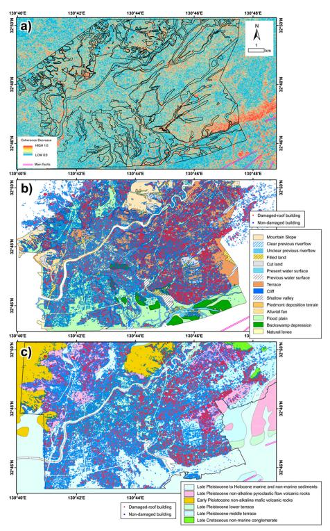
**Figure 4.** Spatial distributions of (a) coherence decrease, buildings covered/non-covered with plastic sheets overlaid (b) on the geomorphological classification map and (c) on the geological map. The locations of these panels are the equivalent of (A) in Figure 1.
