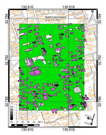
**Figure 8.** Damage detection results for a coherence threshold of 0.3 in the sampled region of Mashikimachi town. Overlapped on Figure 3. Purple colored regions represent the pixels for which the CD values are larger than 0.3.
