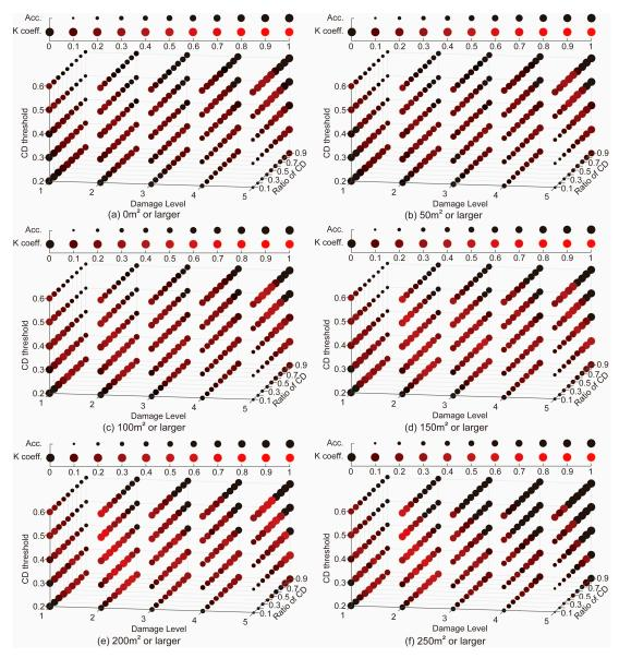
**Figure 7.** Full search results for the overall accuracy and Cohen's Kappa coefficient among multiple DLs (right to left), CD threshold (up to down), and ratio of CD (forward to backward). ( $\mathbf{a}$ – $\mathbf{f}$ ) Building threshold of 0 m<sup>2</sup>–250 m<sup>2</sup> with 50 m<sup>2</sup> intervals. The larger dot indicates the higher accuracy and the brighter red dot shows the higher K coefficient.
