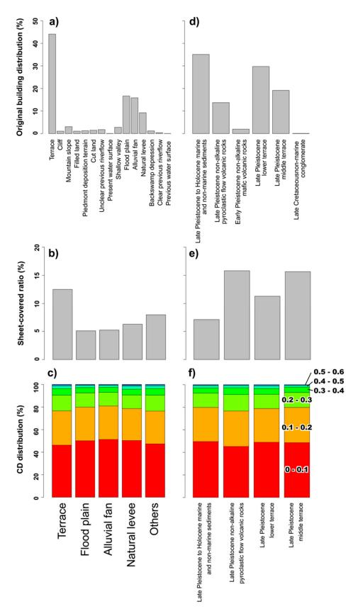
**Figure 5.** (a) Original distributions of entire buildings, (b) sheet-covered ratios, and (c) numerical ratios of coherence decrease (CD) for whole buildings in each geomorphological classification shown in Figure 4c. Those classified into each geological classification (Figure 4b) are shown in (**d**-**f**), respectively. Several classification groups with few buildings are omitted in (**b**,**c**,**e**,**f**).
