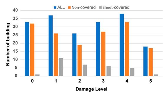
**Figure 9.** Numbers of all, sheet-covered, and non-covered buildings in each damage level in the buildings inventoried in Mashikimachi.
