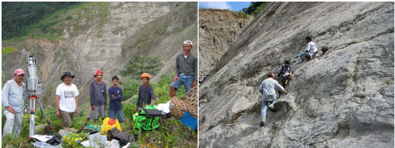
Figure 1. LiDAR survey crew (left) and manual survey crew installing the reflex targets on the slip surface of the February 17, 2006 landslide in Guinsaunon, Southern Leyte, Philippines, photos courtesy Professor Guitierrez and Riegl USA.
