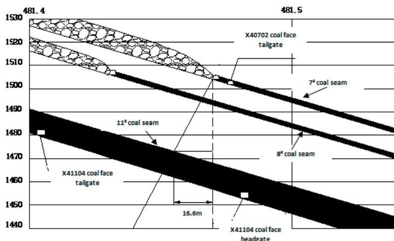
Figure 7. X41104 coal face position.
