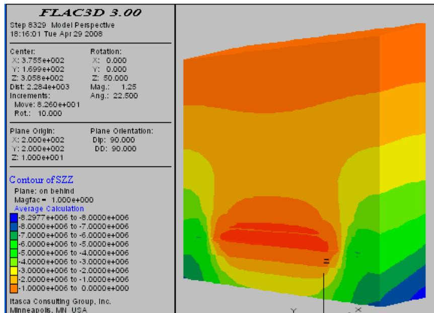
Figure 3. Contour plot of stress in the section along the strike.
