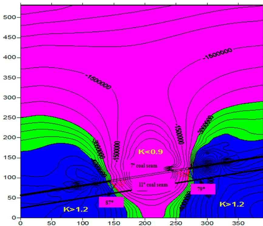
Figure 6. Stress distribution along the dip direction.
