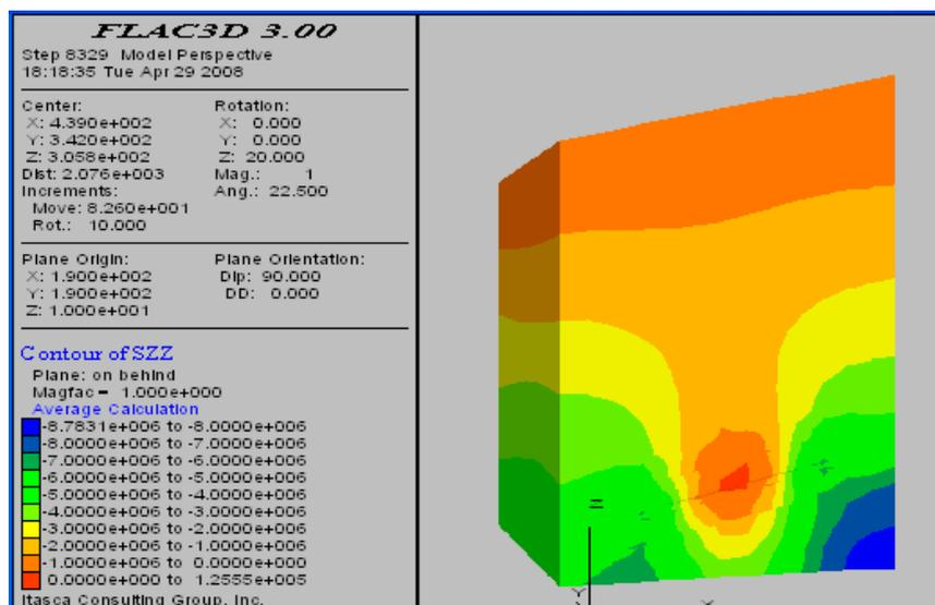
Figure 4. Contour plot of stress in the section along the dip direction.
