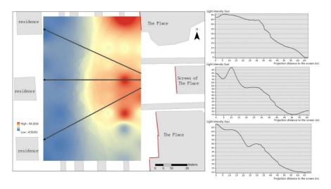
Figure 7. Light intensity distribution at a 1.5-m height.
