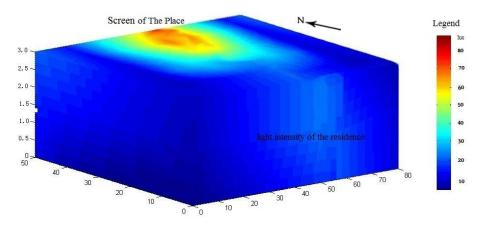
**Figure 6.** The model of the light intensity distribution in the mixed-use zone (sight direction: northwest).
