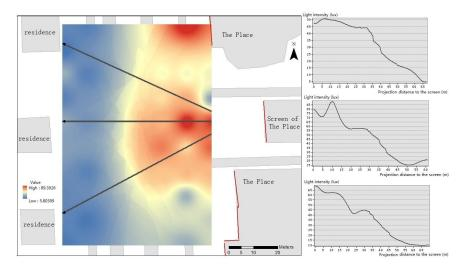
Figure 8. Light intensity distribution at a 3-m height.
