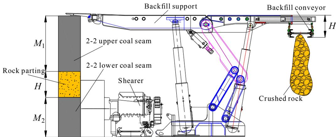
Figure 11. The working state of supports backfilled using crushed gangues.
