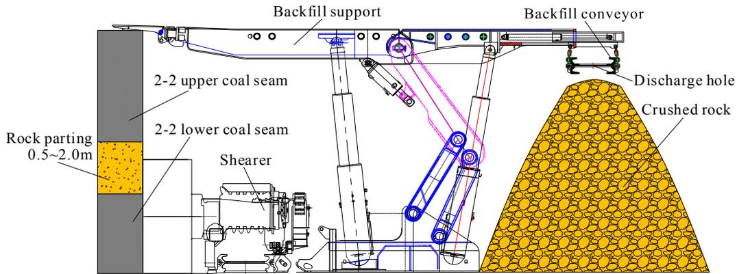
Figure 9. Corresponding working state of the backfill support in Scheme 2.
