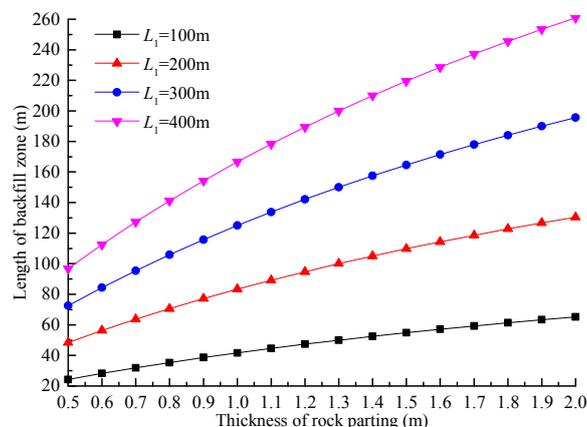
**Figure 14.** Influence of the length of the panel on the length of the backfill zone.
