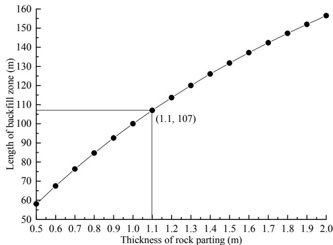
Figure 12. Relationship between the length of the backfill zone and the thickness of the rock parting.
