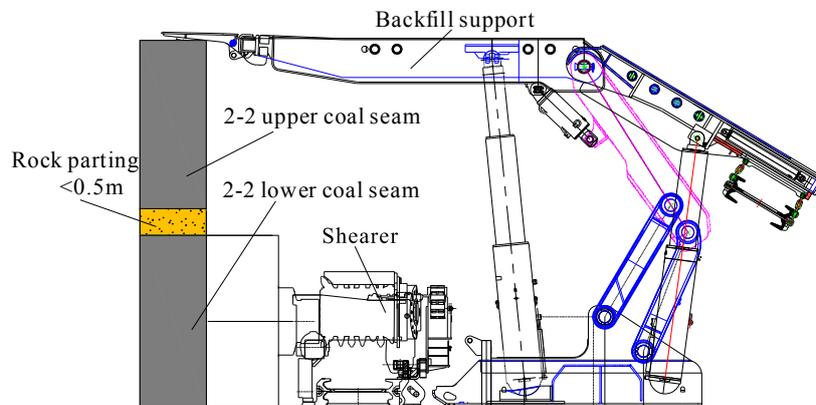
Figure 8. The corresponding working state of the backfill support in Scheme 1.
