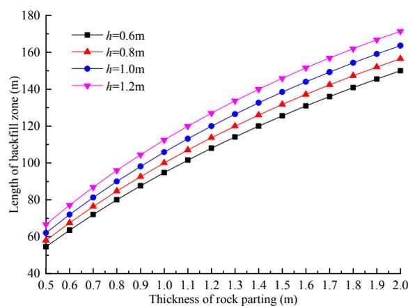
**Figure 16.** Influence of the distance between the bottom and roof of the backfill conveyor on the length of the backfill zone.
