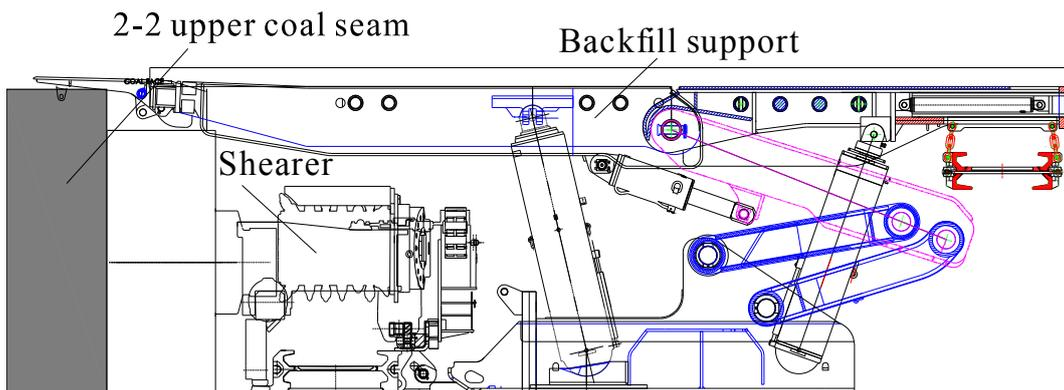
Figure 10. Corresponding working state of backfill support in Scheme 3.
