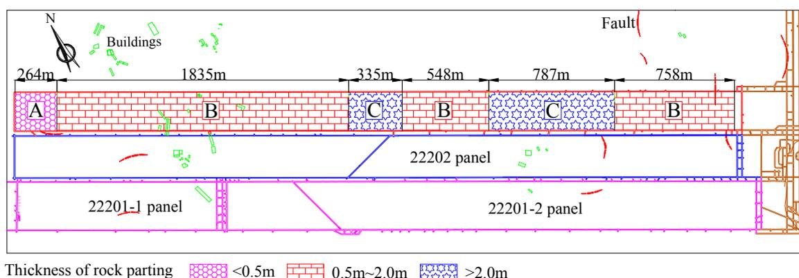
Figure 4. Sub-zones based on the thickness of the rock parting.
