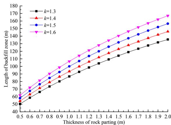
**Figure 13.** Influence of bulking coefficient of rock parting on the length of the backfill zone.
