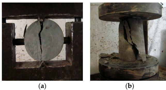
**Figure 3.** Mechanical property testing of rock parting samples. (a) Tensile strength; and (b) compressive strength.
