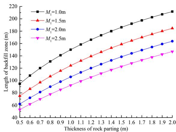
**Figure 15.** Influence of the thickness of the 2-2 upper coal seam on the length of the backfill zone.
