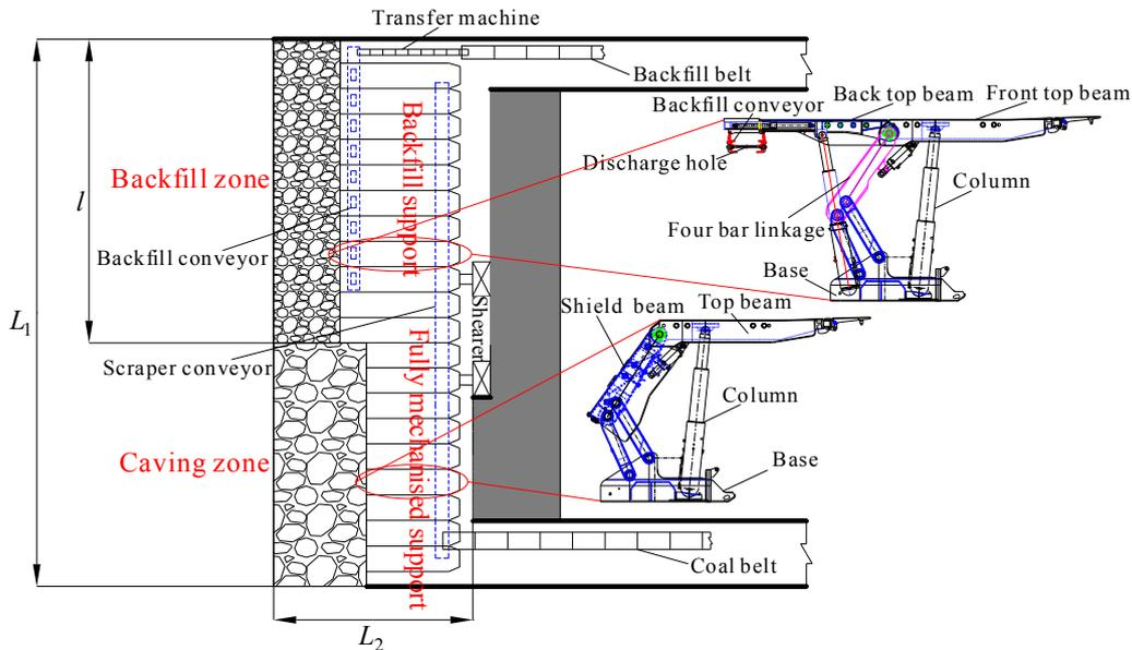
Figure 7. Distribution of devices within the panel.
