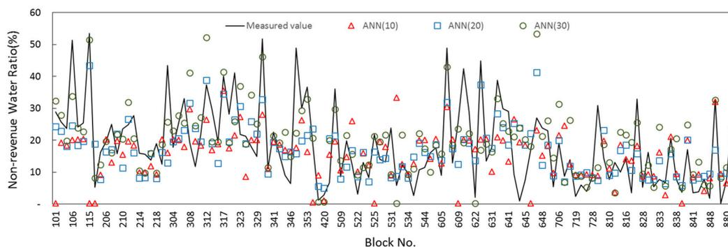
Figure 6. NRW ratio by ANN model simulation in each DMA with outlier removal condition.
