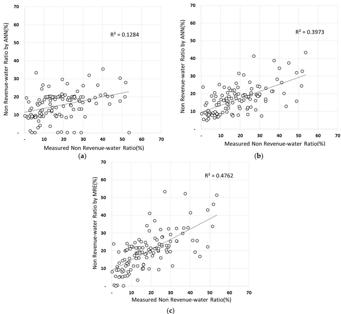
**Figure 8.** Scatter analysis results of NRW ratio with outlier remove condition: (a) ANN using 10 neurons in hidden layer; (b) ANN using 20 neurons in hidden layer; (c) ANN using 30 neurons in hidden layer.
