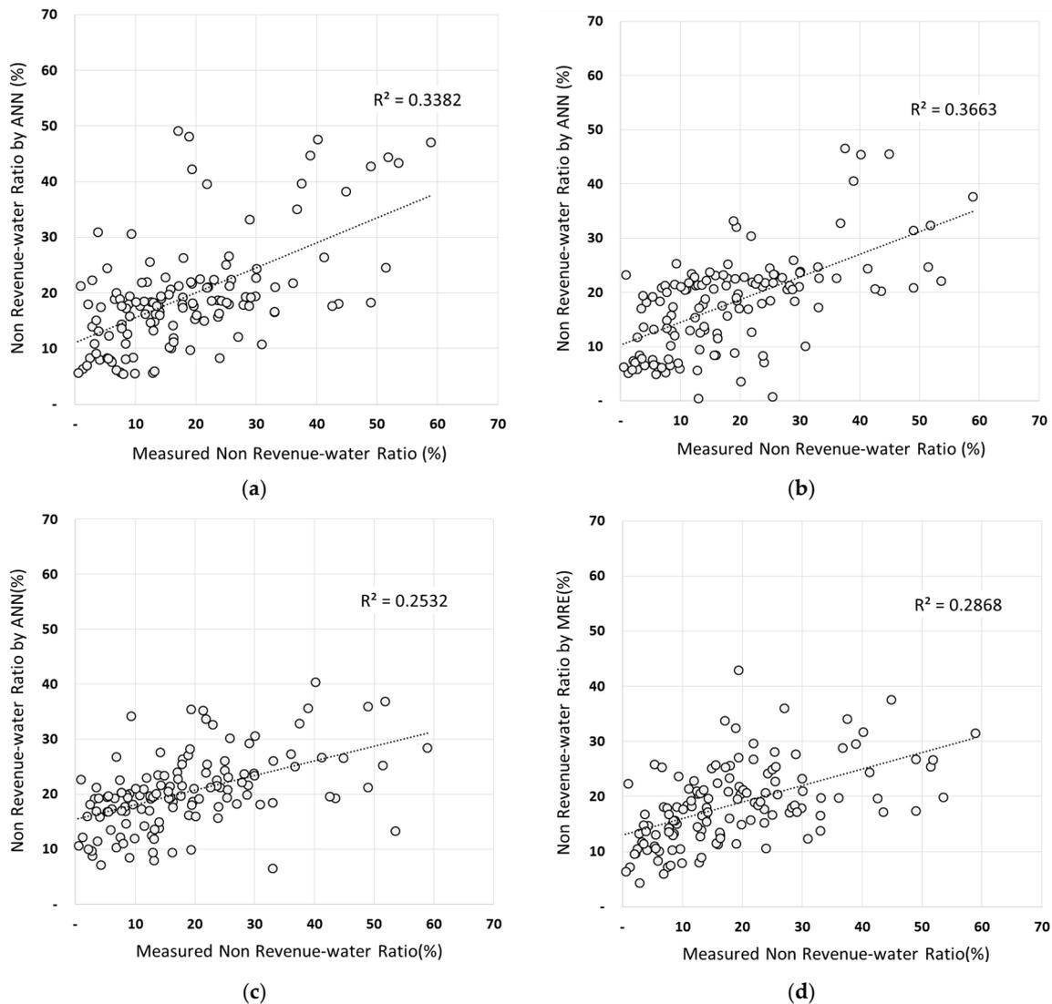
**Figure 7.** Scatter analysis results of NRW ratio: (a) ANN using 10 neurons in hidden layer; (b) ANN using 20 neurons in hidden layer; (c) ANN using 30 neurons in hidden layer; (d) Equation using multiple regression analysis.
