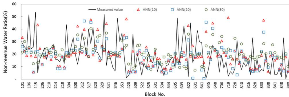
Figure 5. NRW ratio by artificial neural network (ANN) model simulation in each DMA.
