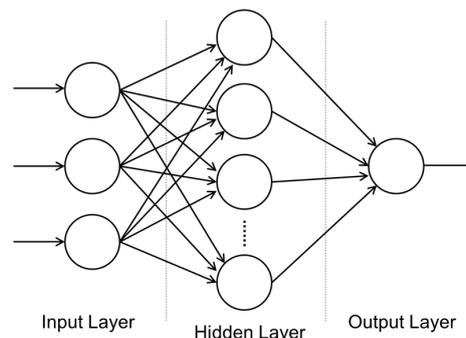
Figure 1. Schematic diagram of multilayer feed-forward neural network [28].
