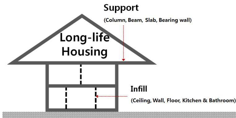
**Figure 3.** Support and Infill of Long-life Housing Concept.
