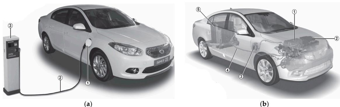
**Figure 1.** Functional diagram of Electric Vehicle and charging machine: (a) 1. Electric Vehicle: SM3 ZE, 2. Standard Charging Cable, 3. Charging Machine: JC 6331; and (b) 1. Electric Motor, 2. 12 V supplementary Battery, 3. Charging Inlet, 4. High Voltage Cable, 5. 400 V Traction Battery [47].
