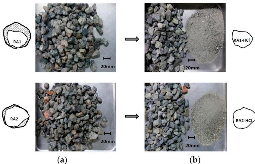
**Figure 6.** RCA samples before and after HCl immersion [18]: (a) before HCl; and (b) after HCl.
