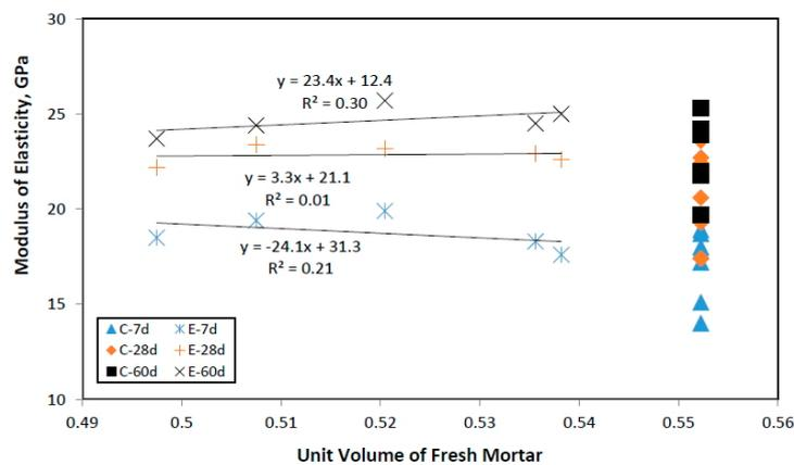
**Figure 12.** Modulus of elasticity results of the concrete with the new mortar volume.
