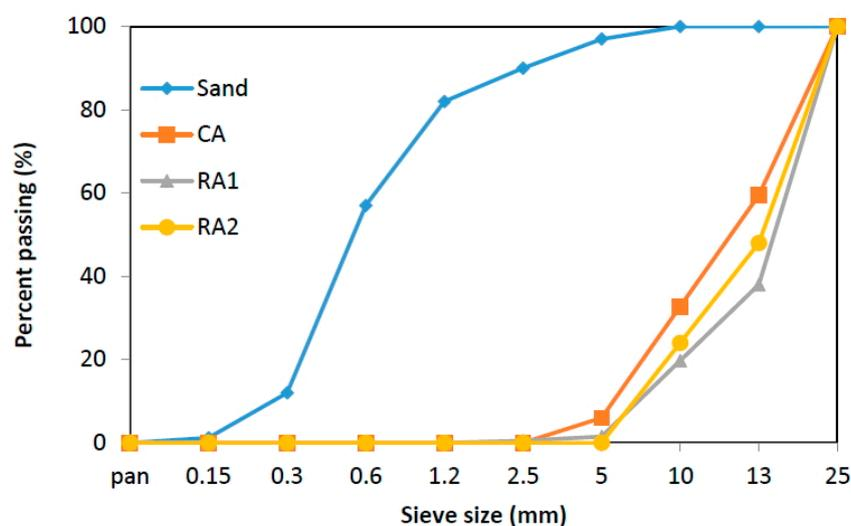
**Figure 3.** Aggregates grading.
