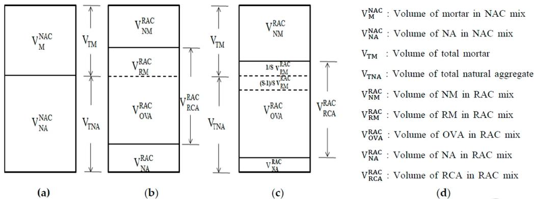
Figure 2. Comparison of various mix design concepts [19]: (a) conventional mix; (b) original EMV mix; (c) modified EMV mix; and (d) notations.
