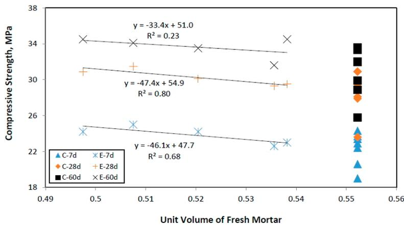
Figure 8. Compressive strength results of the concretes with the new mortar volume.
