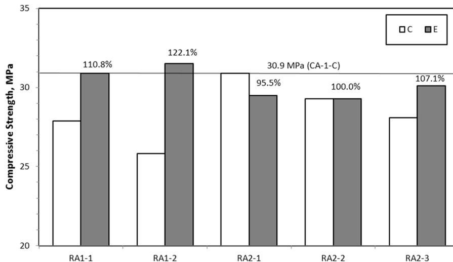
Figure 10. Effect of mix proportioning method on the compressive strength.
