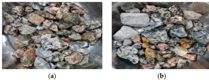
Figure 5. Natural aggregate samples before and after HCl immersion [18]: (a) before HCl; and (b) after HCl.
