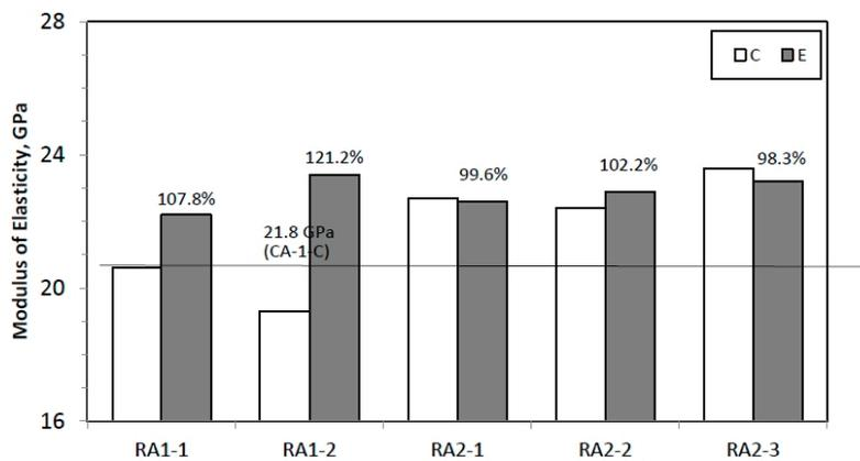
Figure 14. Effect of mix proportioning method on the modulus of elasticity.
