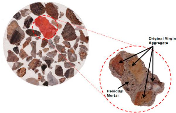
Figure 1. Polished concrete specimen mixed with white cement and coarse RCA only.
