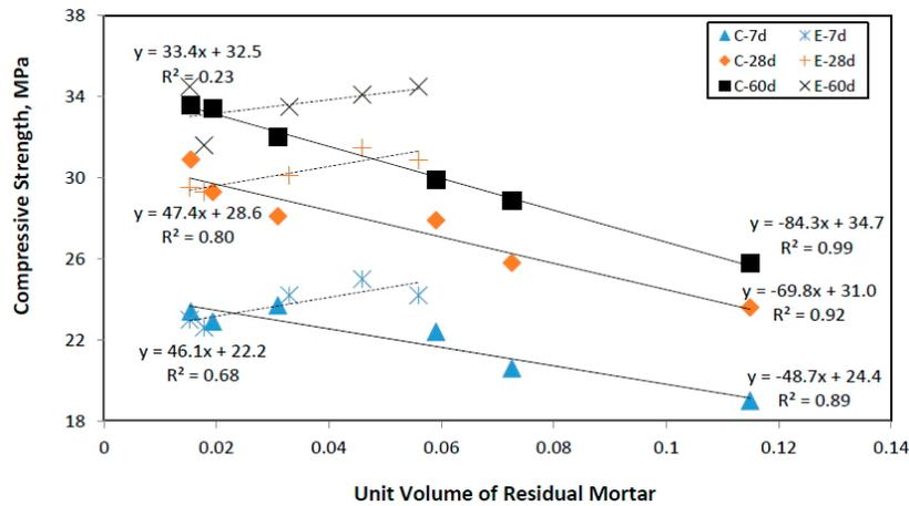
Figure 7. Compressive strength results of the concretes with the residual mortar volume.
