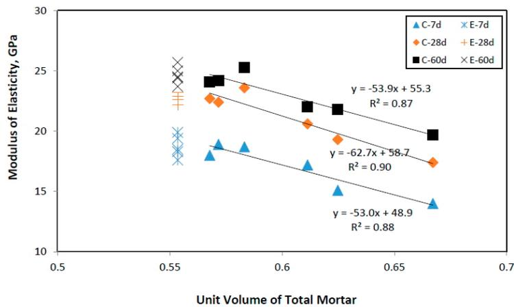
Figure 13. Modulus of elasticity results of the concretes with the total mortar volume.
