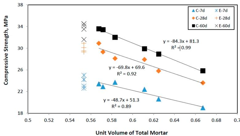
Figure 9. Compressive strength results of the concretes with the total mortar volume.
