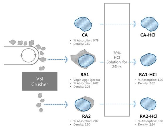
Figure 4. Conceptual illustration of the aggregate treatment process.
