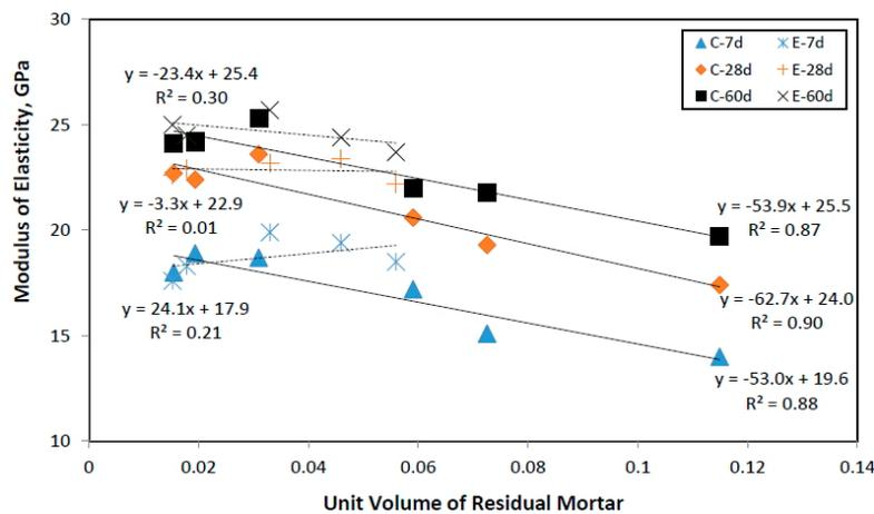
**Figure 11.** Modulus of elasticity results of the concretes with the residual mortar volume.
