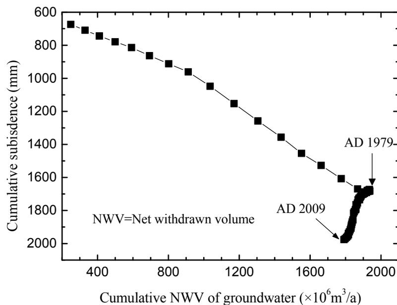
**Figure 3.** Comparison of cumulative land subsidence and NWV of groundwater (based on Reference [25]).
