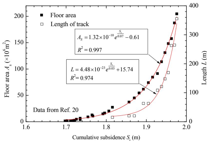
**Figure 5.** Regression analysis of floor area, total length of track in operation and cumulative subsidence.
