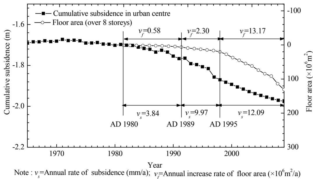
Figure 2. Relationship between floor area and cumulative subsidence (based on Reference [25]).
