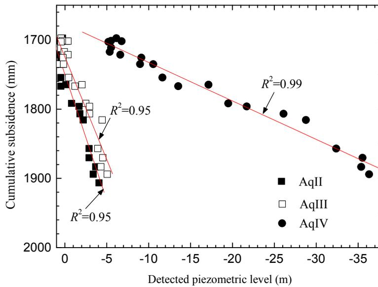
**Figure 4.** Comparison of cumulative land subsidence and detected piezometric level in each aquifer since 1980 (based on Reference [25]).
