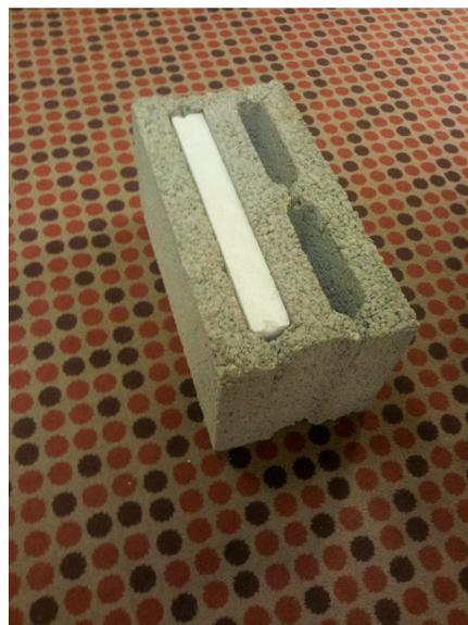
**Figure 1.** Picture of an insulated building block.
