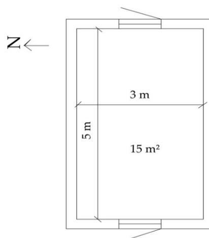
**Figure 1.** Plan of the naturally-ventilated model office with dimensions ( $3.0 \text{ m} \times 5.0 \text{ m} \times 3.0 \text{ m}$ ).
