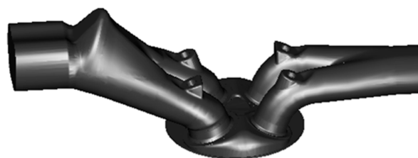
Figure 2. The engine model used for the simulation.
