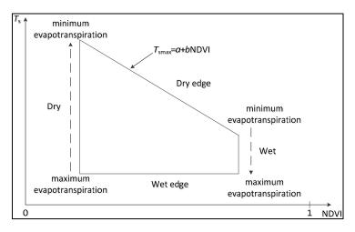
**Figure 4.** Definition of the TVDI. The TVDI for a given NDVI is estimated using  $T_s$ ,  $T_{smin}$  and  $T_{smax}$  (see Equation (2)).
