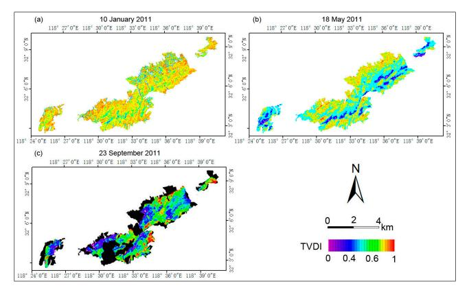
**Figure 6.** Spatial distribution of the TVDI for the three scenes. On 23 September 2011, the area covered by cloud was screened out and is represented in black in Figure 6c.
