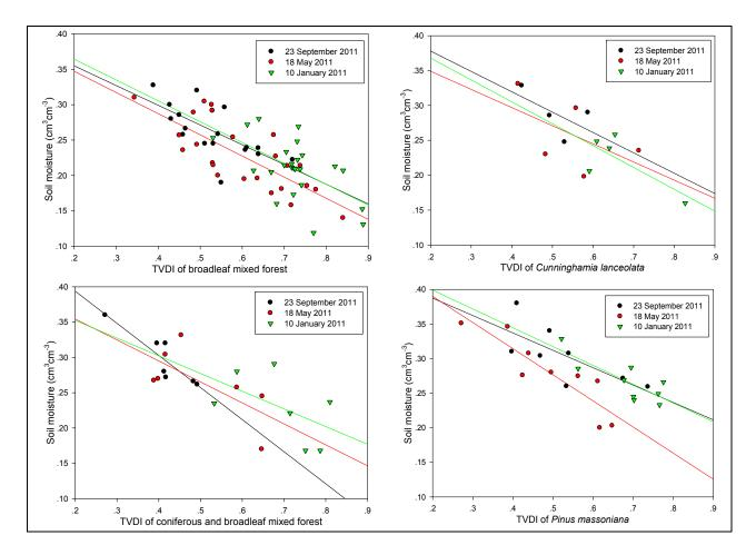
**Figure 7.** Comparison of the TVDI with the observation points of *in situ* soil moisture measurements for each land cover on 10 January 2011, 18 May 2011 and 23 September 2011.
