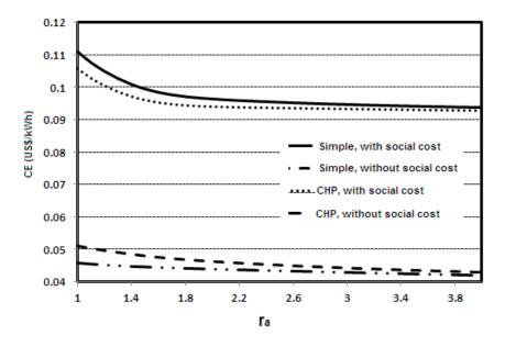
**Figure 7.** Variation of electricity cost (with and without inclusion of the external cost of air pollution) with excess air ratio for a simple and CHP IC engines at an inlet air temperature of 15 °C.
