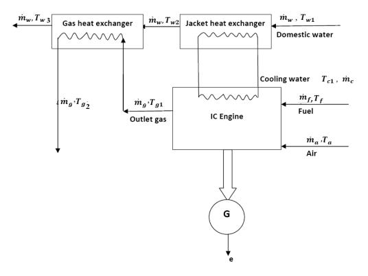
Figure 1. Configuration of the system.
