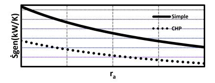
**Figure 6.** Variation of entropy generation with excess air ratio for simple and CHP internal combustion engines at an inlet air temperature of 15 °C.
