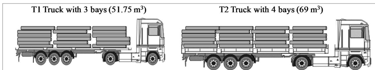
Figure 3. Types of truck based on real volume capacity for pulpwood.
