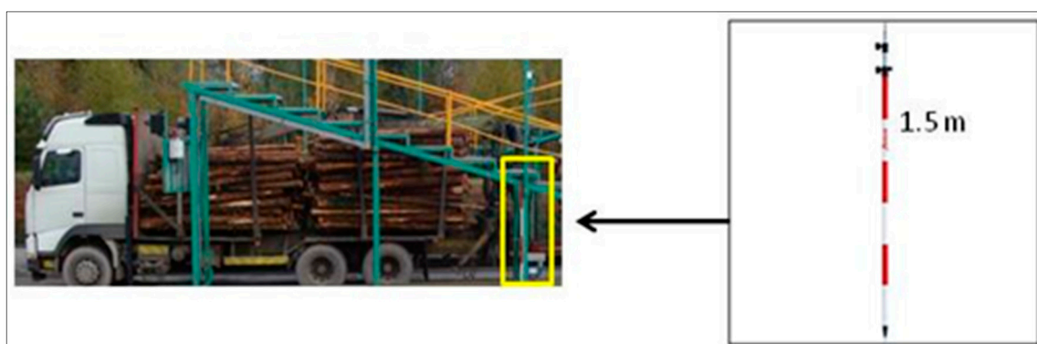
Figure 2. Location of the measuring staff for scaling.
