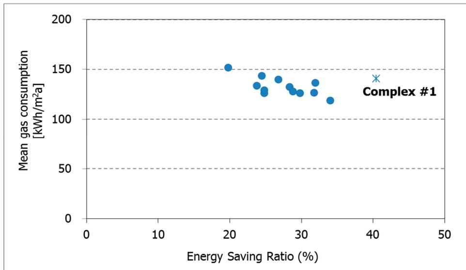
Figure 10. Energy saving ratios and gas consumptions in the individual heating complexes.
