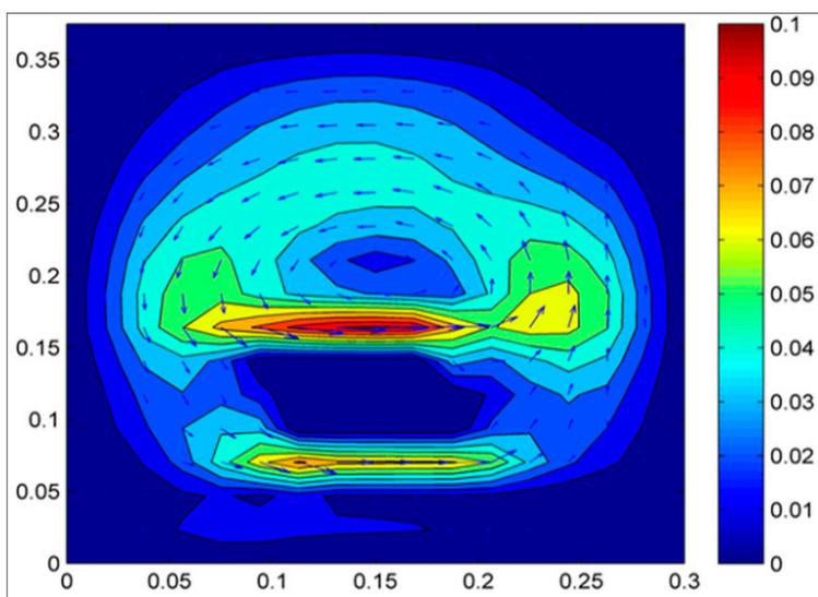
**Figure 9.** Two-dimensional flow velocity contours for an impeller speed of 400 rpm.
