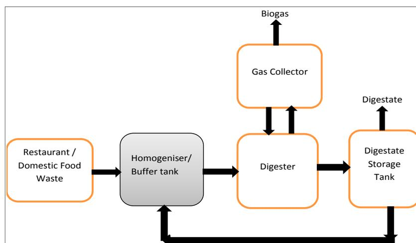
In a continuous processing system, digesters are equipped with a preparation tank where various substrates are mixed and prepared for loading [2]. The feedstock production, storage and supply are important parts of the bio-mass to bio-energy conversion chain [5]. In an organic waste biodegradability
