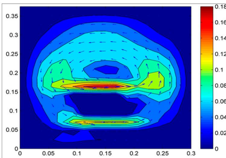
**Figure 10.** Two-dimensional flow velocity contour for an impeller speed of 500 rpm.
