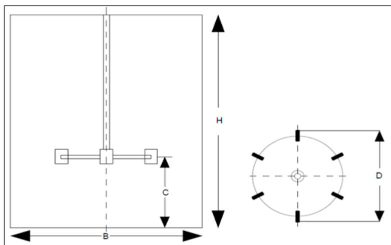
The properties of carrot-orange soup used in the simulation are listed in Table 1. An impeller of diameter 0.16 m is used in the simulation. Other properties of the impeller and tank are provided in Tables 1 and 2 [11].
