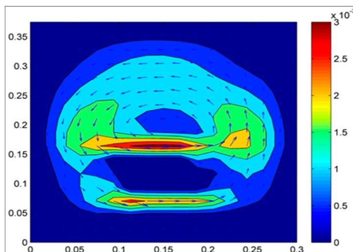
**Figure 6.** Two-dimensional flow velocity contour for an impeller speed of 100 rpm.
