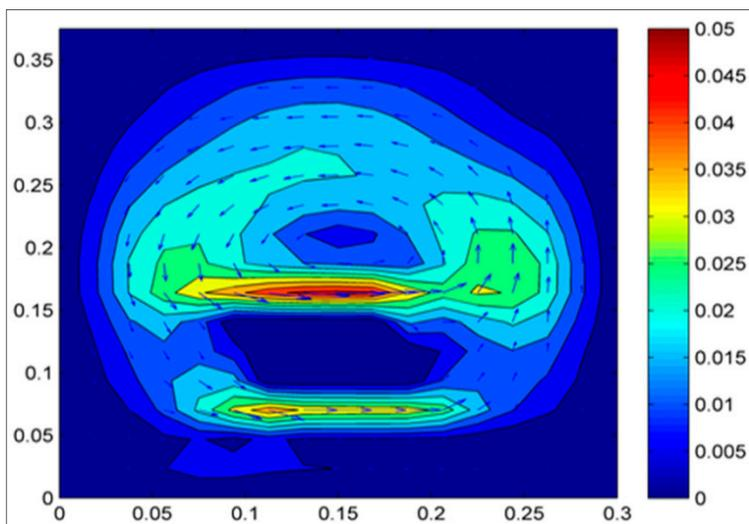
**Figure 8.** Two-dimensional flow velocity contour for an impeller speed of 300 rpm.
