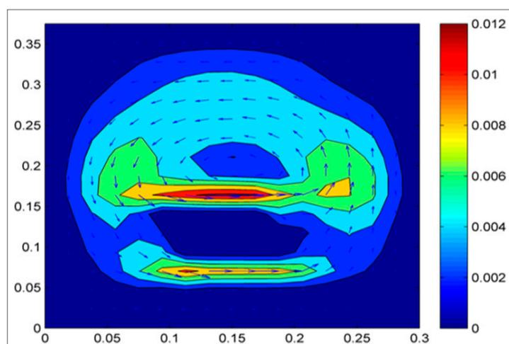
**Figure 7.** Two-dimensional flow velocity contour for an impeller speed of 200 rpm.
