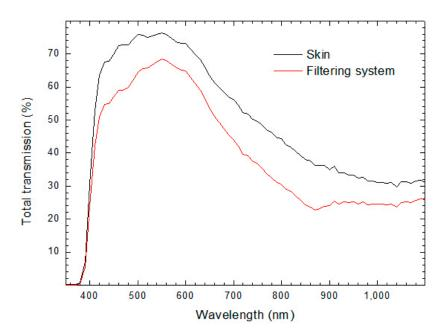
Figure 8. Skin and filtering system total transmission spectra.
