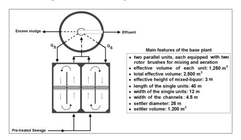
Figure 1. Modified base plant used for the tests.
