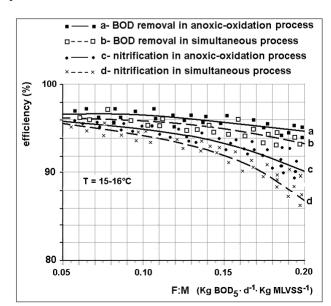
Figure 7. Efficiency of BOD<sub>5</sub> removal and of nitrification for the two processes studied.
