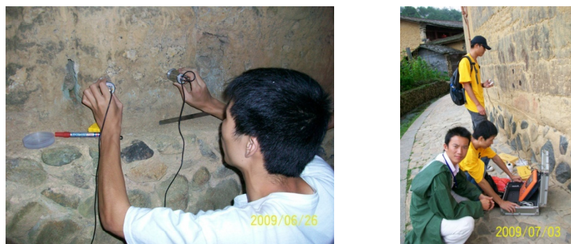
Figure 5. Ultrasonic testing heads and device.
