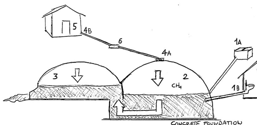
In Figure 1 a basic sketch of a biogas plant Camartec design is given. The plant consists in the following parts:
