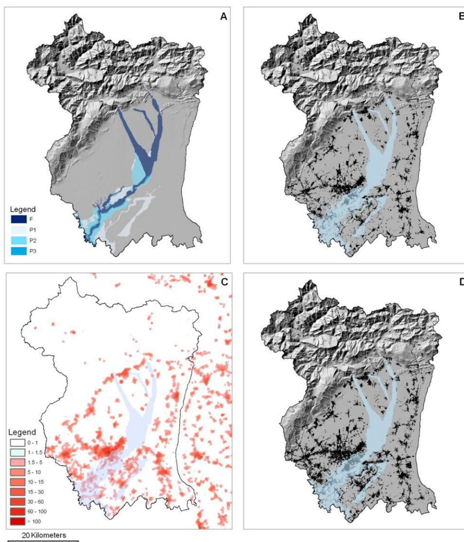
The hazard areas defined in the flood hazard map are the result of a two-step approach. First, the areas prone to a 100-year flood event are mapped. Second, the extent of the areas is verified by using a bi-dimensional flood model and historical flood records. In the flood hazard areas water depth could
