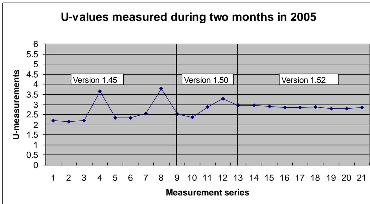
Note: Versions relates to software development. The Version 1.52 compared to version 1.45 and 1.50 include an updated radiative model and an adjusted measuring procedure which secure a better acclimatization of the heat absorption sensor.
