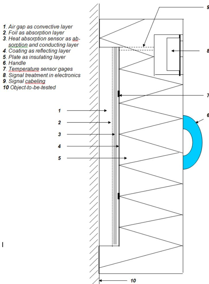
The temperature of the heat absorption sensor is measured continuously over a short period of time, and from the relative increase of energy the U-value can be calculated. The system is separated from the surrounding environment with a highly insulating material {5}, of low thermal diffusivity and low conductivity.
